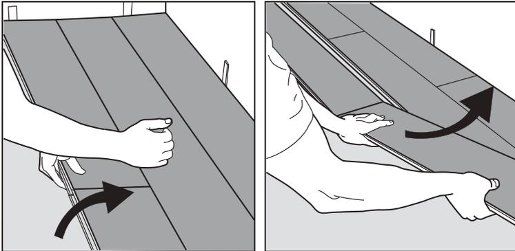
Separate the whole row by lifting it up delicately at an angle. To separate individual plank end-joints within a row, rotate the plank upward to disassemble.
