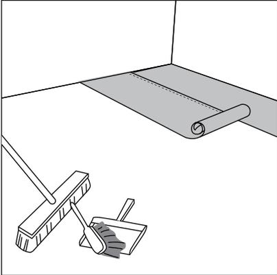
① Thoroughly clean the subfloor before you start the installation. If you are installing over a concrete subfloor, a minimum 6-mil plastic poly sheeting must be added prior to flooring installation. Run the moisture barrier in the same direction as the flooring planks. The barrier should be butted side-by-side with no overlap. Tape seams together.
