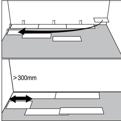
⑤ Start the second row with the leftover cut part of the last plank of the previous row. This small plank should measure at least 12" (30cm). Otherwise, use another plank that should be cut in two. Short pieces should be cut to at least 12" (30cm).
