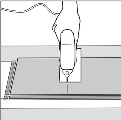
④ If cutting with a jig saw, the laminate surface should be turned down. If cutting with a hand saw, the laminate surface should be face up.
