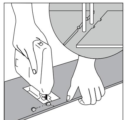
**9** Holes for pipes: measure the diameter of the pipe and drill a hole that is 7/8" (20mm) larger into the plank. Saw the plank into two pieces perpendicular to the length and bisecting the previously drilled hole. Then lay the two pieces in place around the pipe.
